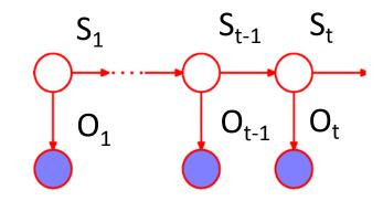
$$= p(O_t|S_t = k) \max_i p(S_t = k|S_{t-1} = i)V_{t-1}^i$$
